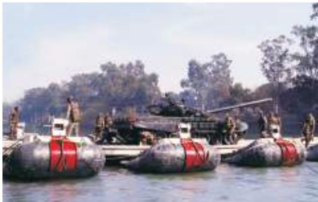
Float Assembly for KM Bridge
